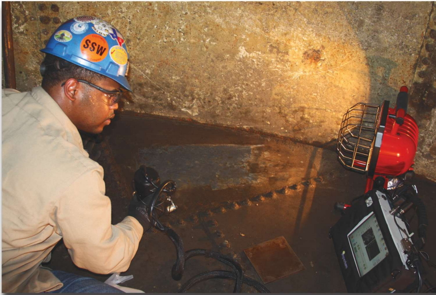
An inspector scans the bottom of a storage tank with the acoustic video imaging system. Photo courtesy of Imperium, Inc.
